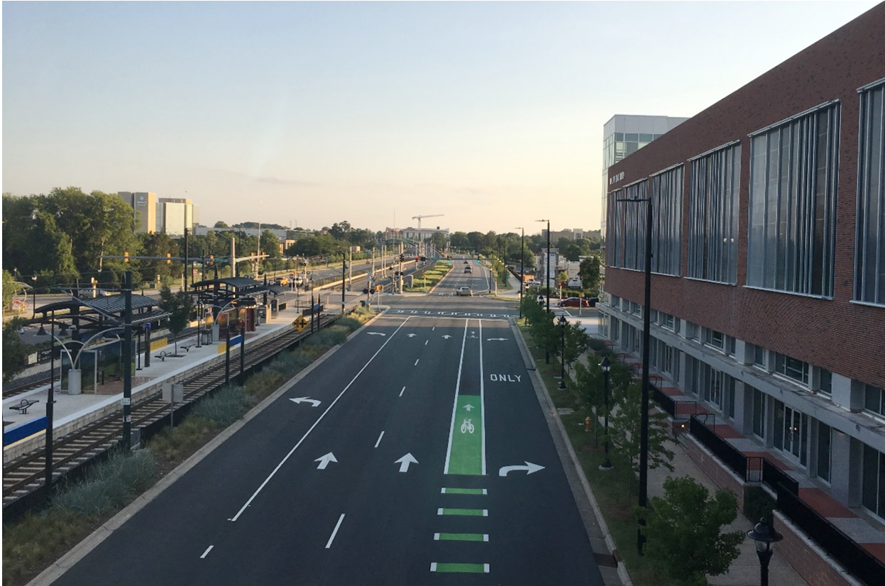
Figure 2. Green colored pavement used to designate bike lane and mixing zone. Source: FHWA.
