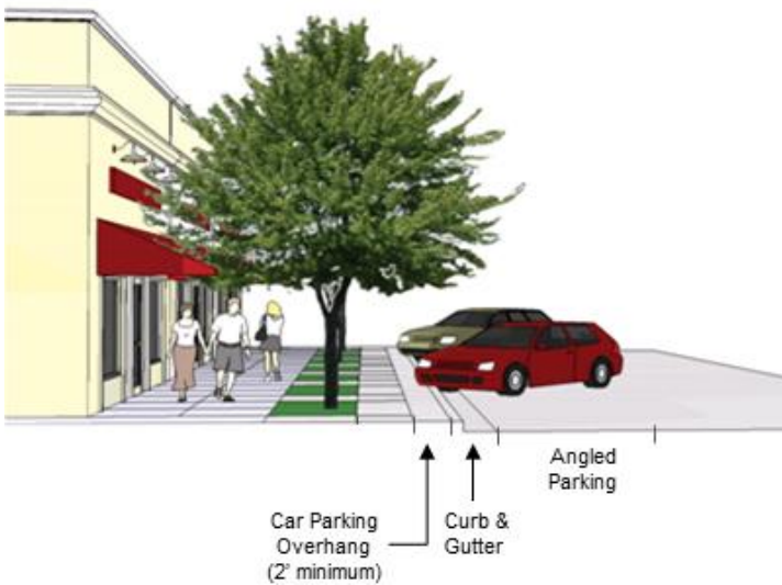
Source: Jacksonville Design Guidelines and Best Practices Handbook (Section 1: Commercial Development) Figure 2.2-5 Angled parking diagram
