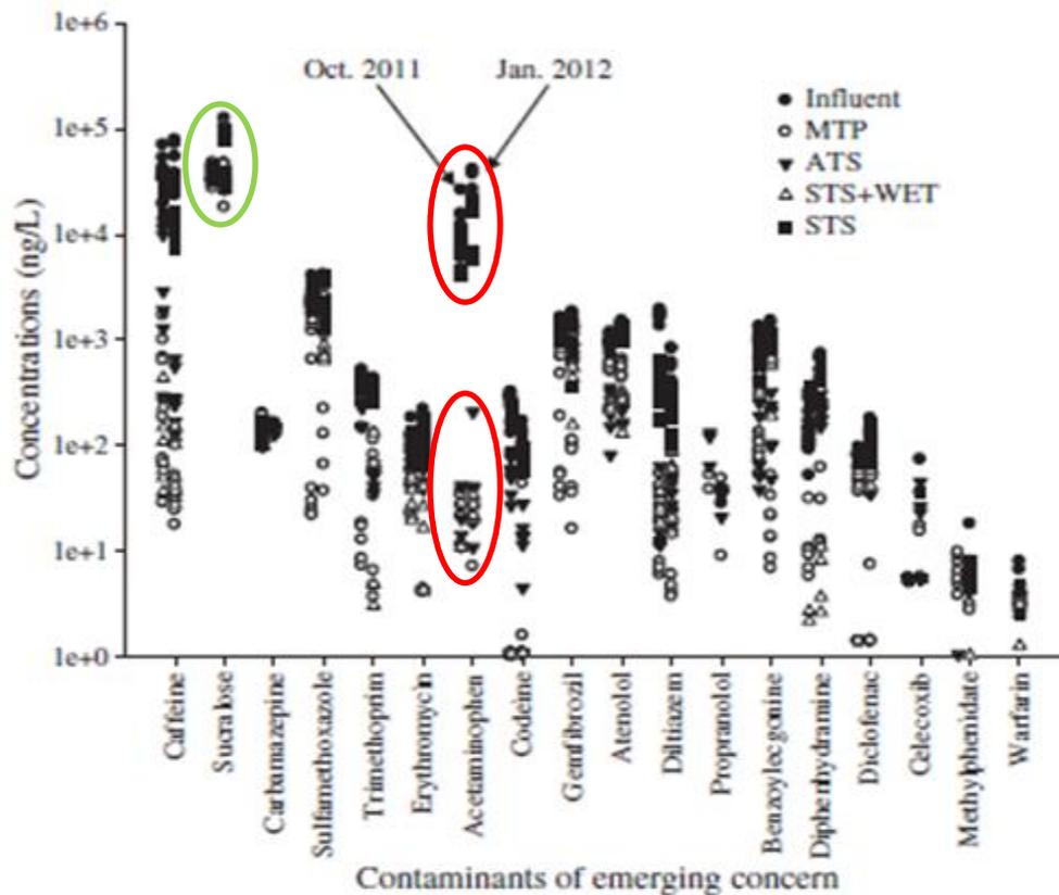
**Fig. 2.** Detected target contaminants of emerging concern in influent and various effluent discharges by season. MTP = municipal treatment plant; ATS = aerobic treatment system; STS = septic treatment system; WET = wetland.
