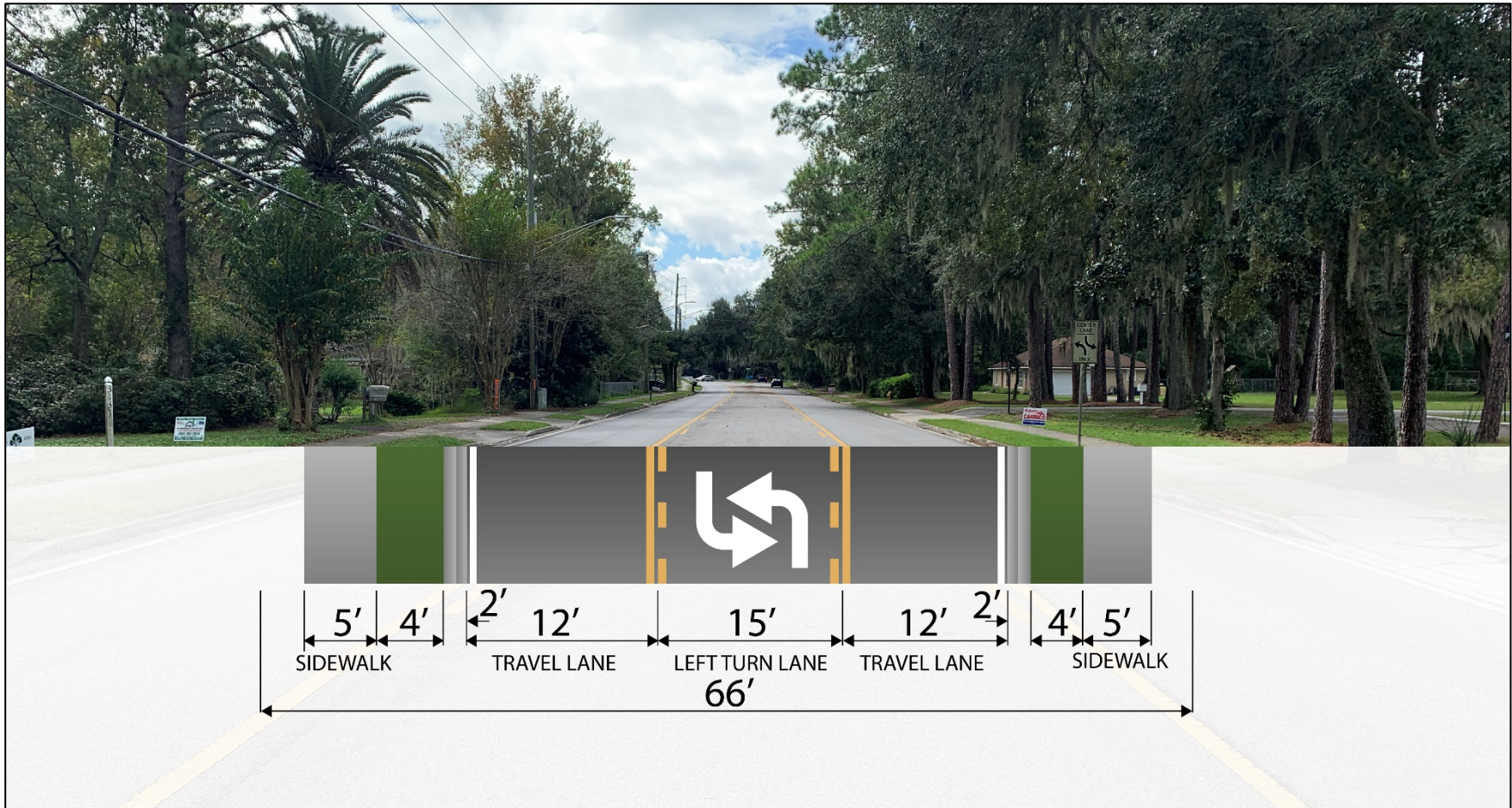
FIGURE 2-6 TYPICAL SECTION: SOUTH OF STARLING AVENUE
