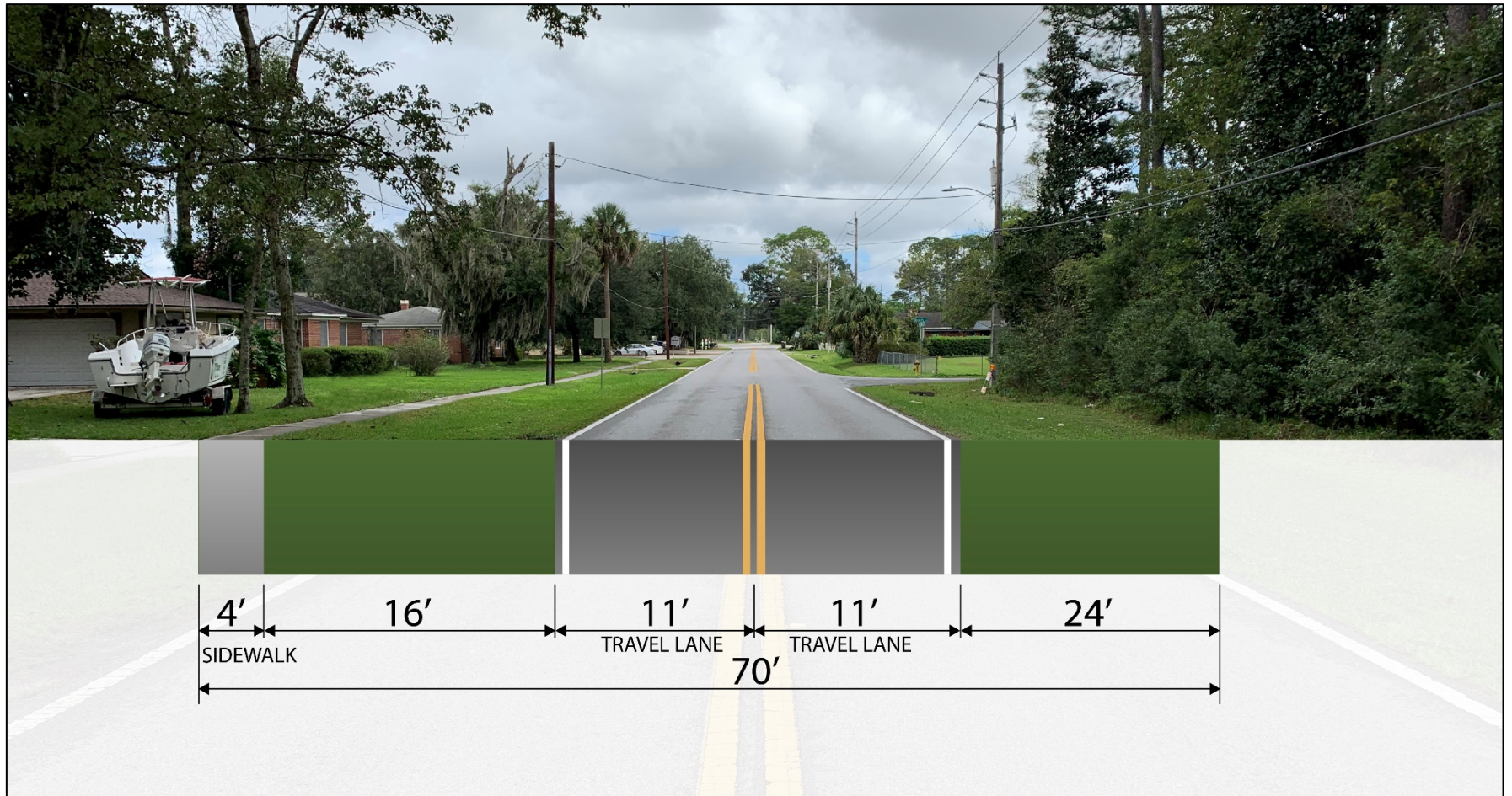
FIGURE 2-5 TYPICAL SECTION: SOUTH OF IBACH ROAD
