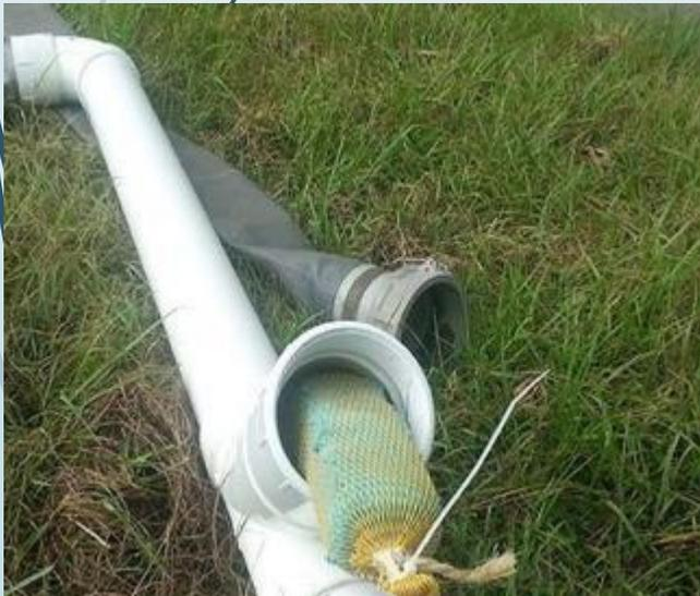
The link manifold is designed to eliminate the need for open dewatering ditches and allow for water treatment in-line with anionic polyacrylamide(PAM).
