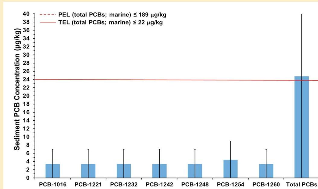
Mean concentrations of individual PCB congeners and total PCBs in sediments collected in 2017. Probable Effect Level (PEL) is indicated by the dotted red line. Threshold Effect Level (TEL) is indicated by the solid red line.
