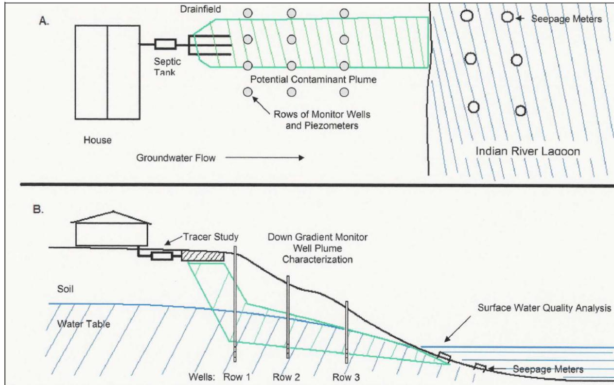
Figure 1. Typical Monitoring Set-Up
