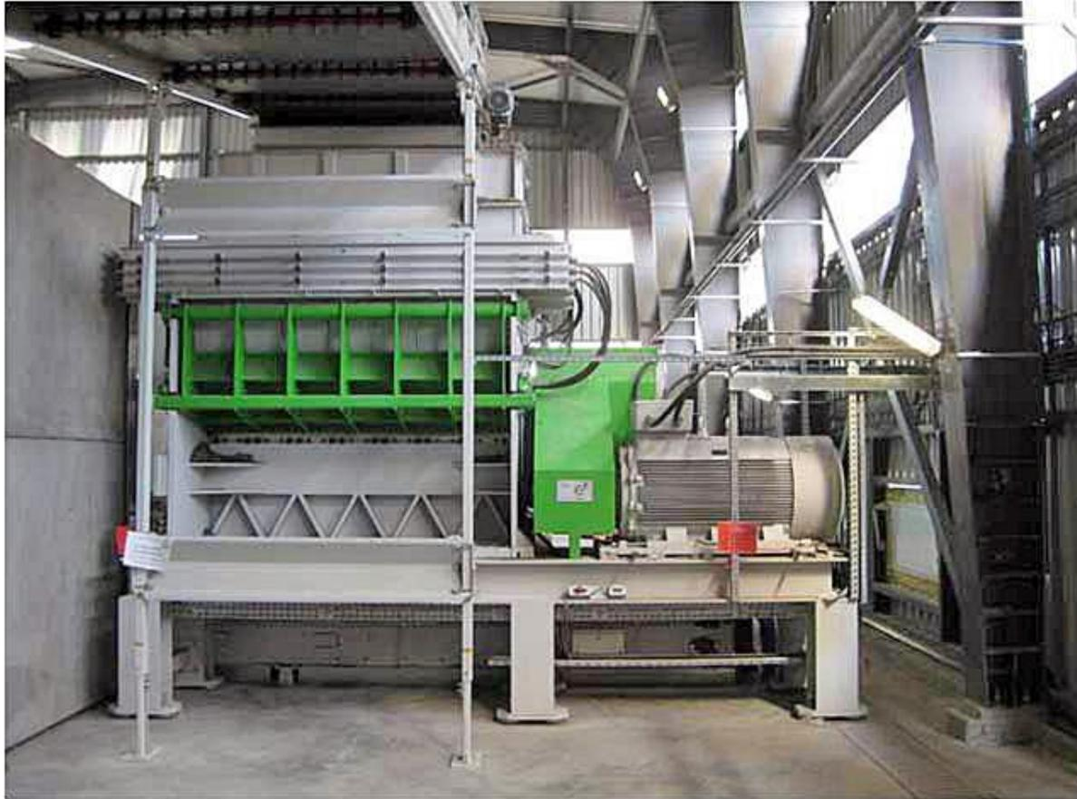
**Fine Cut (secondary) Shredder
