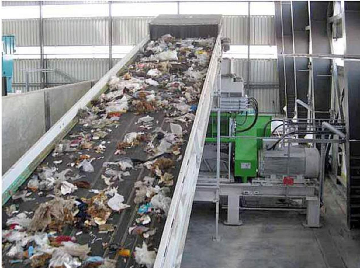
**Discharge Conveyor to Fine Cut Shredder
